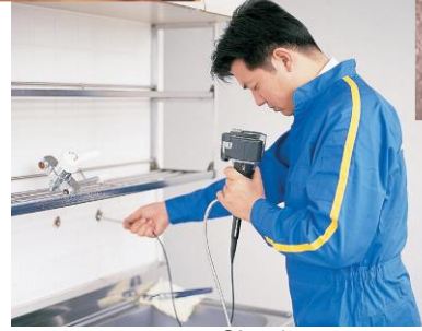
<Checks on water pipes and drainpipes>
