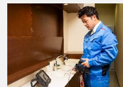
Water Pipe Inspection Using a Video Scope
