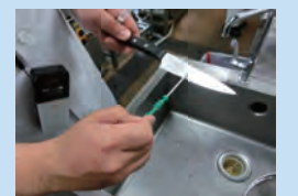
ATP wipe inspection (to confirm cleanliness)
