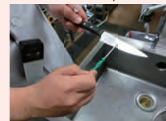
ATP wipe inspection (to confirm cleanliness)
