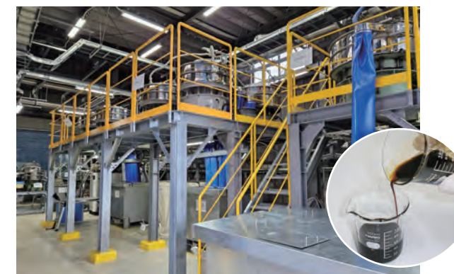
“Recycled Oil Bio,” a heavy-oil alternative fuel produced by separating and recovering only the oil from waste liquid generated by restaurants and food factories. In March 2024, the production line was expanded to double its capacity. In January 2025, it received the Chairperson’s Award from the New Energy Foundation at the FY2024 New Energy Awards.
